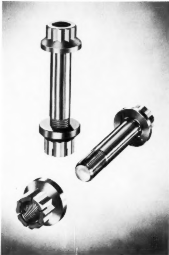
EWB-22 Bolt is Entirely New. External wrenching head with increased bearing area permits great preloading without indentation of bolted surface. New thread form, generous fillet under head, smooth overall surface increase tensile strength and fatigue resistance.
